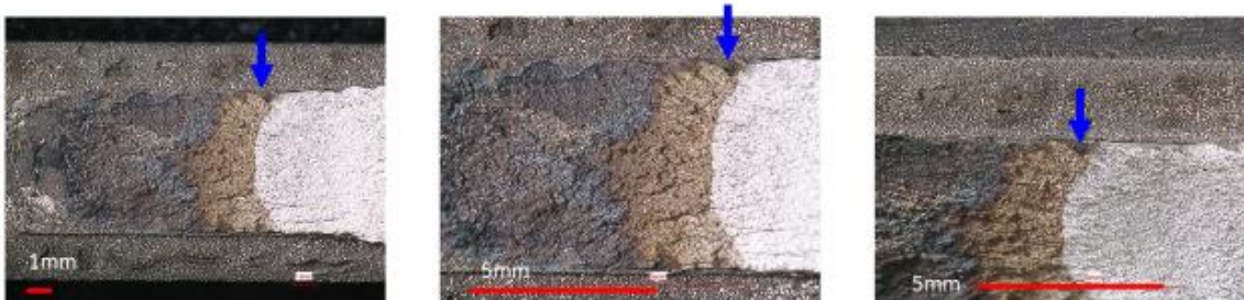
Blue arrow: The representative of edge crack revealed by low-angle illumination
