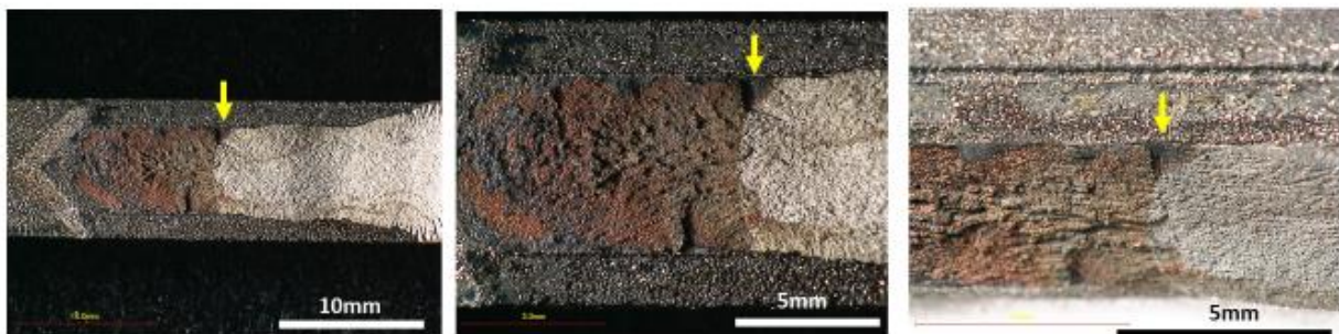
Invalid test specimen in accordance with 11.6.1 e) sub clause 3
