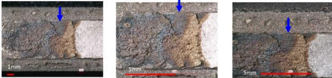
Blue arrow: The representative of edge crack revealed by low-angle illumination
